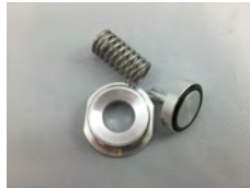
Differential valve components. (Do not put these into Cleaning Station)
